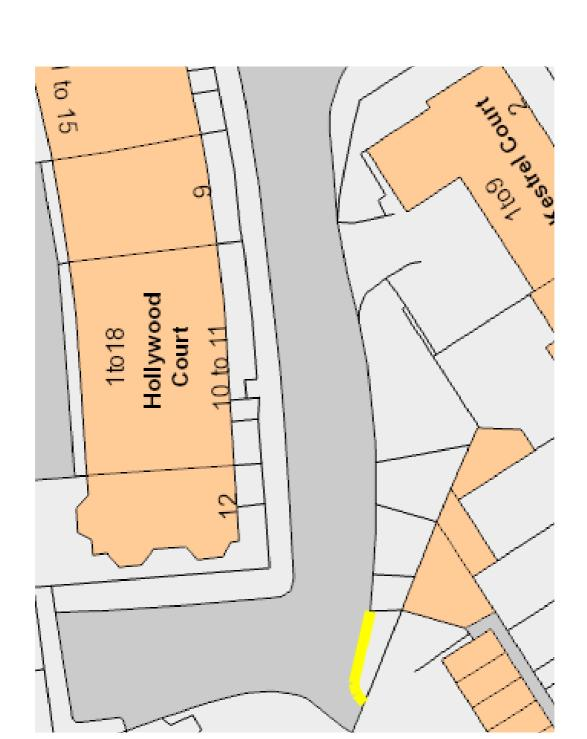
Install DYL on the southern side at a point 67 meters from the junction with Canterbury Road for a distance of 4 meters
